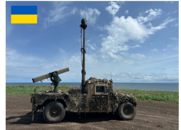
VAMPIRE –R150 gimbal integrated with the APKWS 70mm laser-Guided Rocket System
