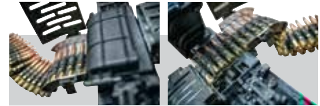
Dual feed system for fast ammunition switching
